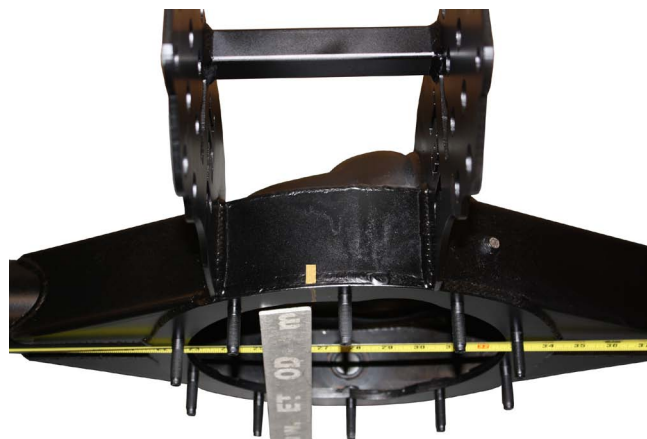
B- Mark the top and bottom of the housing.
