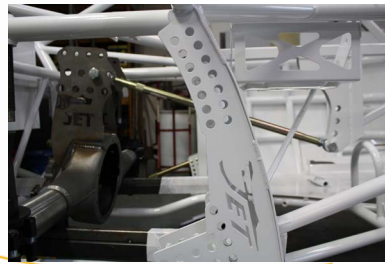
P - Torque Link or Solid Pull Bar located in the bottom hole on the frame bracket.
