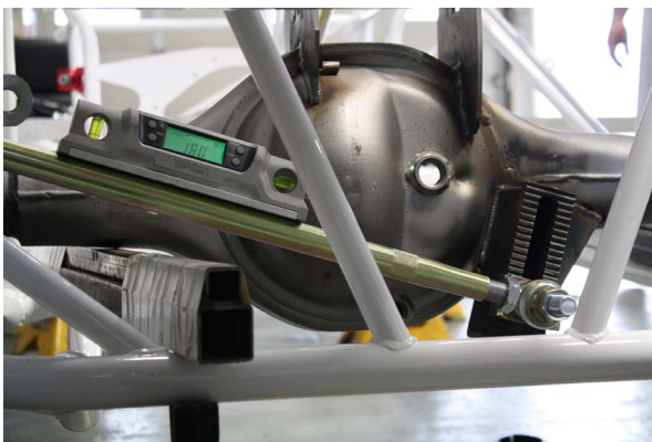
I - Using an angle finder to check the angle of the panhard bar. Start at 18°.
