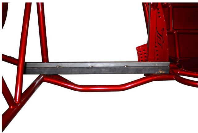
D- Ride height block on left lower frame rail underslung.
