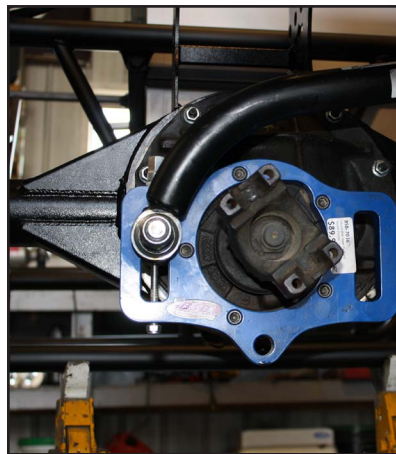
H - Putting the J-bar in the center of the Pinion Plate
