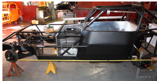
L - Measure from the lower ball joint zerk to the front of the rear end housing on cars 2008 & older
