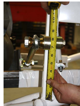
J- Mount the pan-hard bar bracket at 6 1/2" up from the bottom rail to the bottom of bracket.
