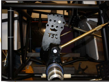
N - Pull Bar located in the middle-third hole on the rear-end housing
