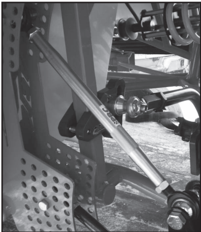
G - Installing the J-Bar in cars #532 and Newer
